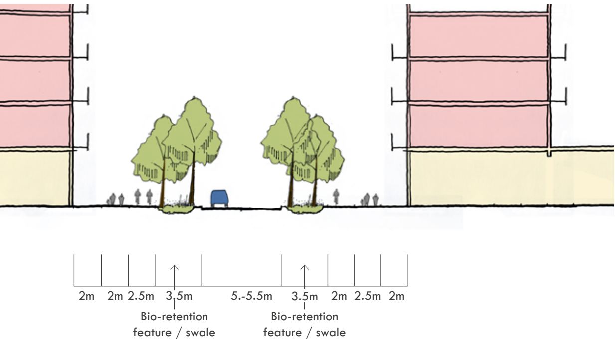
Fig.46: Main street access section
